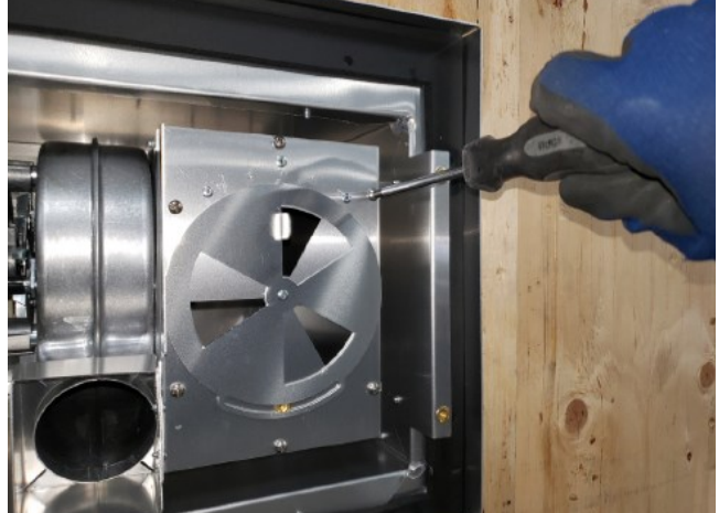
Figure 8.2 - Exhaust Assembly Screws
