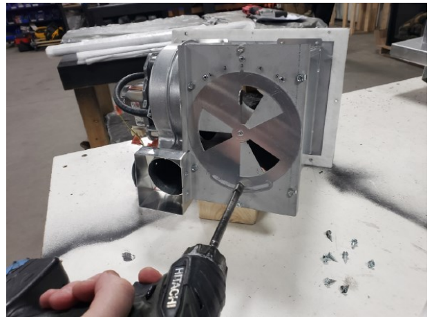
Figure 2.4 - Loosen Locking Screw
