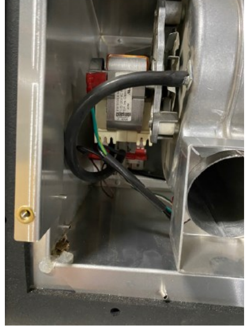
Figure 8.8 - Screws Securing Vacuum Switch Bracket
