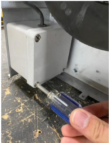
Figure 4.2 - Remove Electrical Box Lid
