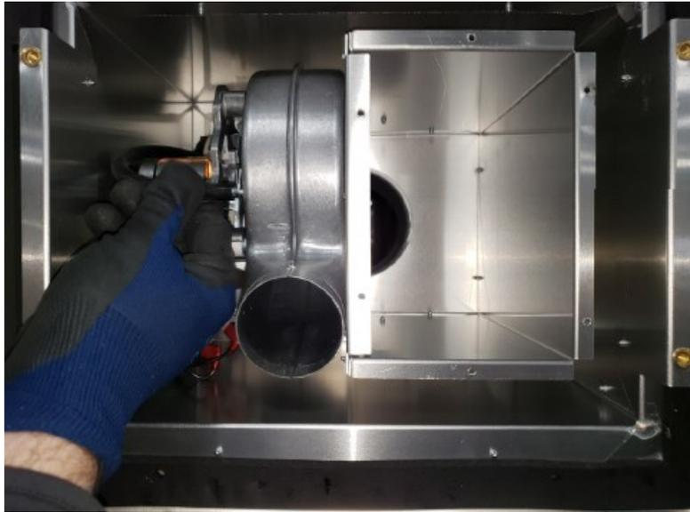
Figure 8.5 - Remove Vacuum Tube
