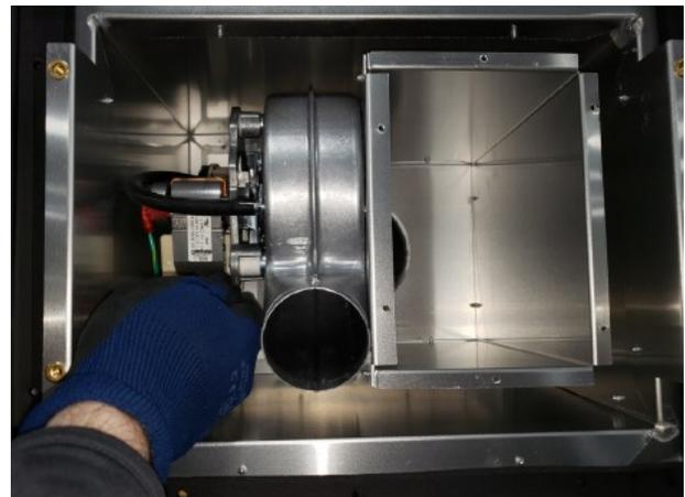
Figure 8.4 - Remove Hot, Neutral, and Ground Wire
