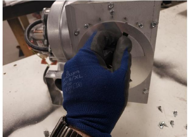
Figure 2.5 - Adjust the Draft Bypass
