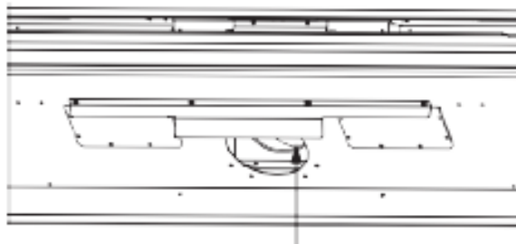
Insert Restrictor Plate Into Exhaust Pipe in Firebox Ceiling with Tabs Facing Towards You.
