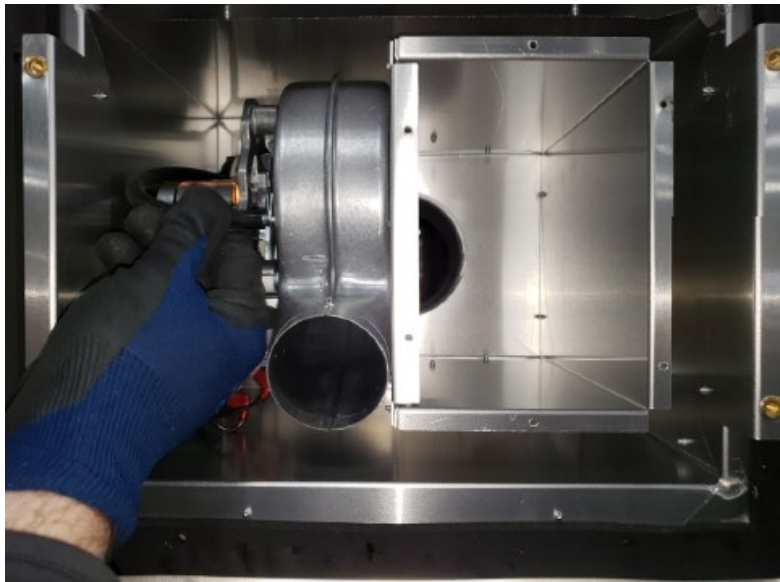
Figure 8.5 - Retirer le tube d'aspiration
