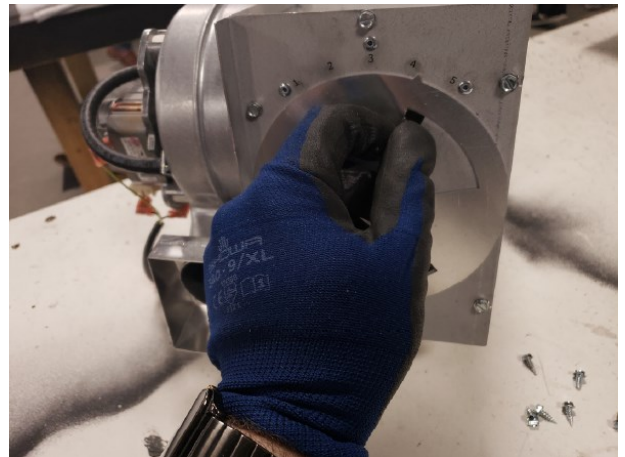
Figure 2.5 - Adjust the Draft Bypass
